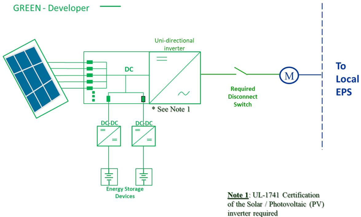
**Figure 4: DC coupled ESS (Configuration 3)**
