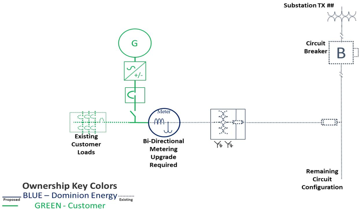
**Figure 1: Typical Layout for Net Metering DER < 250 kW**
