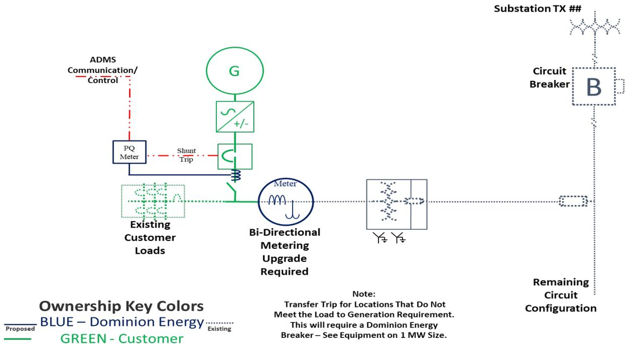
**Figure 2: Typical Layout for Net Metering DER  $\geq 250$  kW and  $< 1,000$  kW (No DTT required)**
