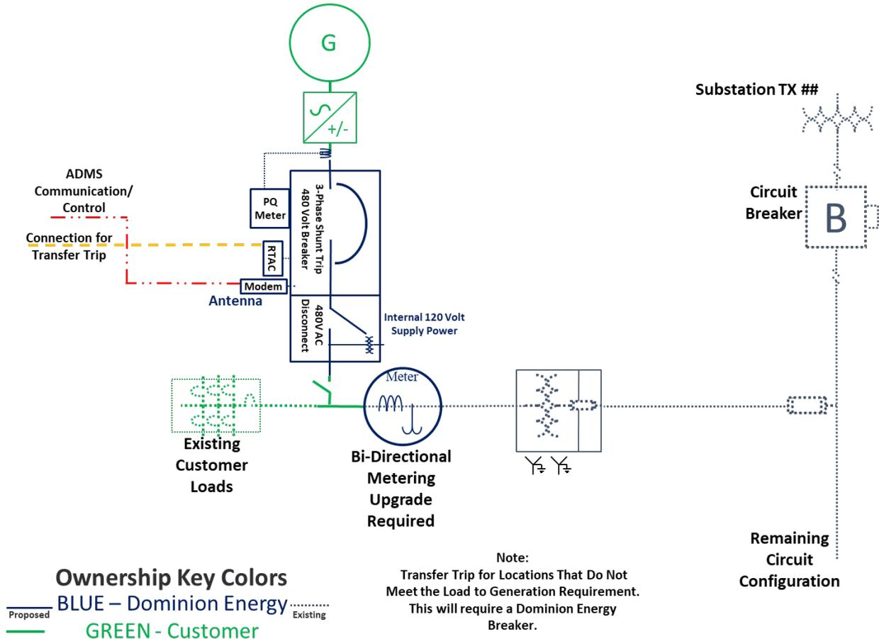
**Figure 3: Typical Layout for Net Metering DER  $\geq 250$  kW and  $< 1,000$  kW (DTT Required)**
