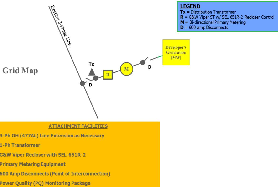
**Figure 2: Typical Primary Distribution Facility Layout with additional details (DER customer owned transformer)**
