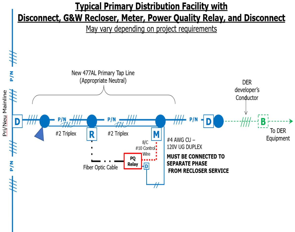
**Figure 3: Typical Primary and Secondary Distribution Facilities Layout (Dominion owned transformer)**
