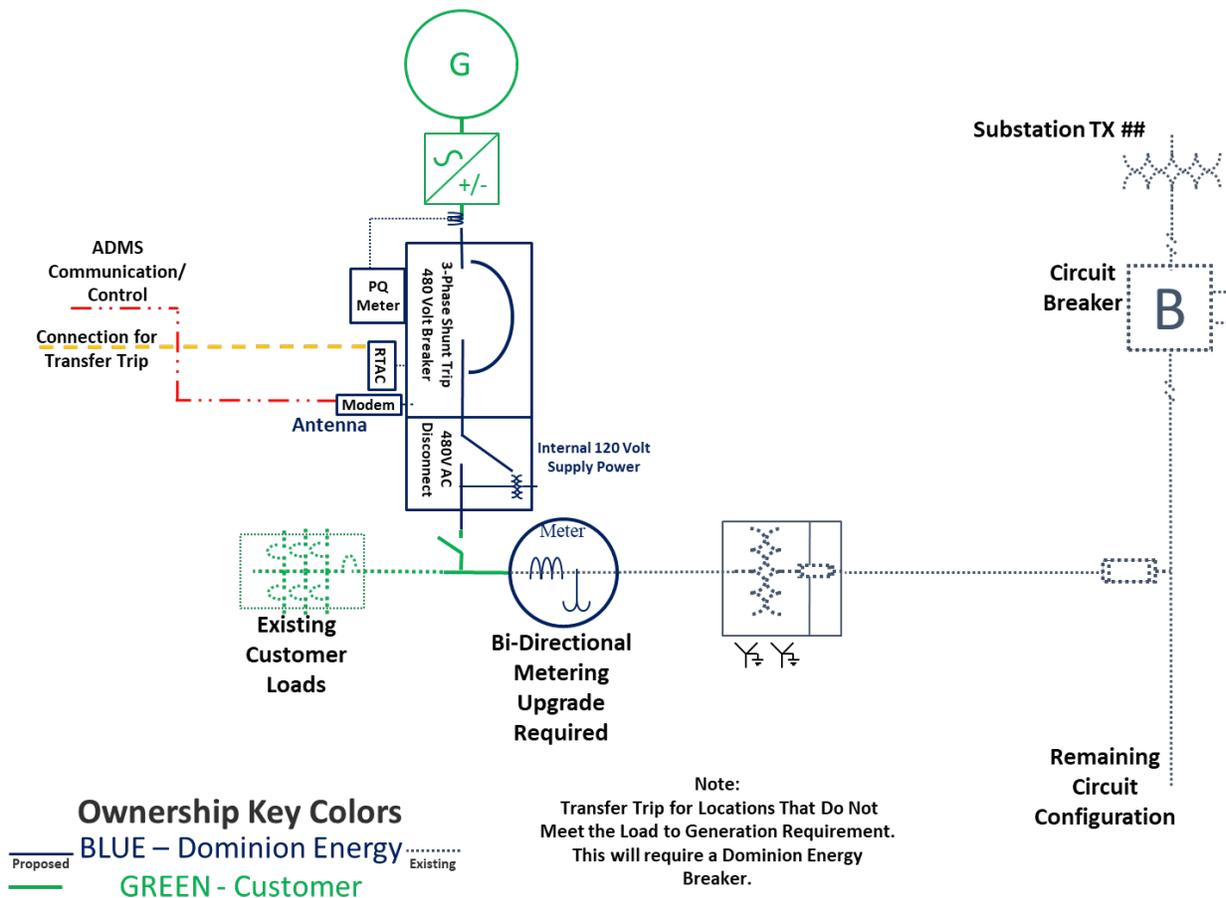
**Figure 4: Typical Layout for Net Metering DER  $\geq 1,000$  kW and  $\leq 3,000$  kW (Existing Service Transformer)**
