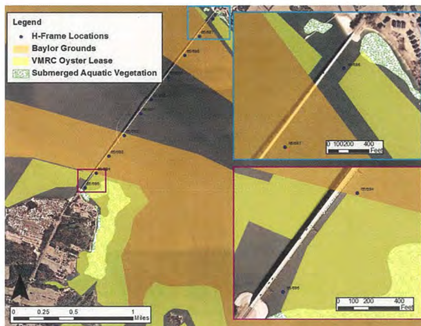
Figure 3.1-2. Illustration of Overhead Alternative construction components which will incur sediment impact overlaid on environmental resources. Note that the indicators for location of the H-Frame and Piles are not to scale as they would not be viewable at scale. The insets shown illustrate zoomed views near the north and south shoreline demonstrating that the structure locations do not fall within the VMRC Oyster Lease areas.
