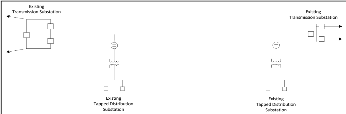
Figure 5. Existing Transmission Line
