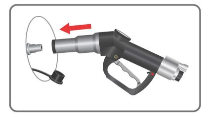
Place the fueling nozzle onto the receptacle until it stops.
