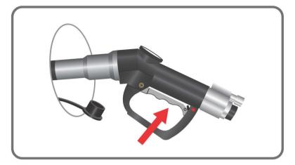
2 Hold the fueling nozzle steady and retract the trigger slightly until it snaps in. Begin refueling.
