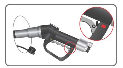
After refueling, release the latch in direction of the arrow.
