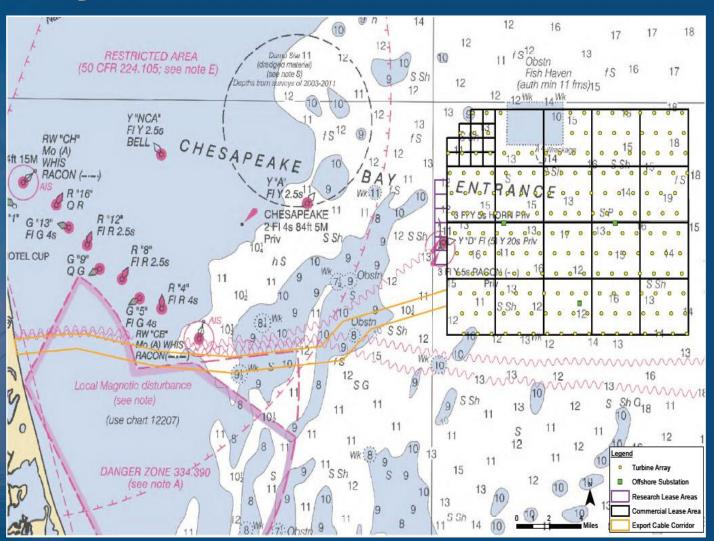
The Offshore Project Area, including the Lease Area and the Export Cable Corridor. The proposed wind farm layout contains turbines spaced 0.7 nm by 0.9 nm.
