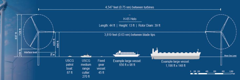
Depiction of different types and sizes of vessels and aircraft between two wind turbines, spaced 0.7 nm by 0.9 nm. These vessel and aircraft graphics have been drawn to scale to more accurately demonstrate transportation navigation and clearance between turbines.
