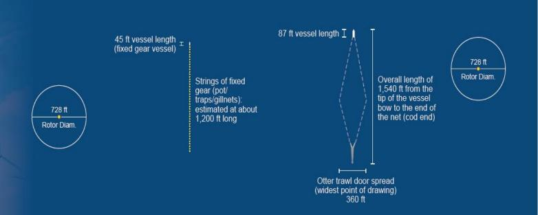
Depiction of different types of fishing equipment (fixed gear and trawl) between two wind turbines, spaced 0.7 nm by 0.9 nm. These fishing equipment graphics have been drawn to scale to more accurately demonstrate fishing equipment navigation between turbines.
