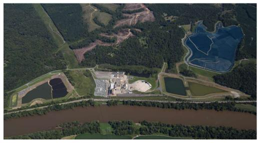
Approximately 6.2 million cubic yards of Bremo CCR material is consolidated and stored in the North Ash Pond under a temporary rain cover. The full rain cover is designed to prevent dust and keep rainwater out of the pond while the material is in storage.
