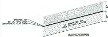
24" LOW PERMEABILITY SOIL LINER - ALT #2 GCL UNDERLAIN BY 24" SOIL LINER 1x10-5 CM/SEC N.T.S. 6 D-1
