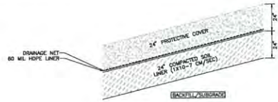
24" LOW PERMEABILITY SOIL LINER - OPTION #1 24" SOIL LINER 1x10-7 CM/SEC N.T.S.
