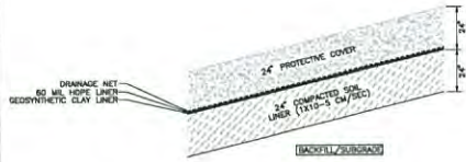
24" LOW PERMEABILITY SOIL LINER - OPTION #2 GCL UNDERLAIN BY 24" SOIL LINER 1x10-5 CM/SEC N.T.S.
