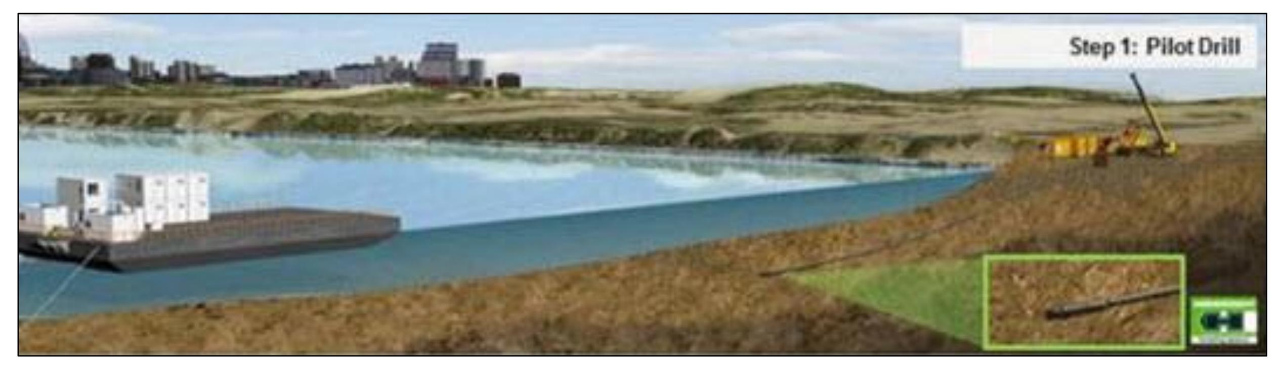
Pilot Drill - the initial boring is completed by pushing and rotating the drill pipe along a predetermined path.
