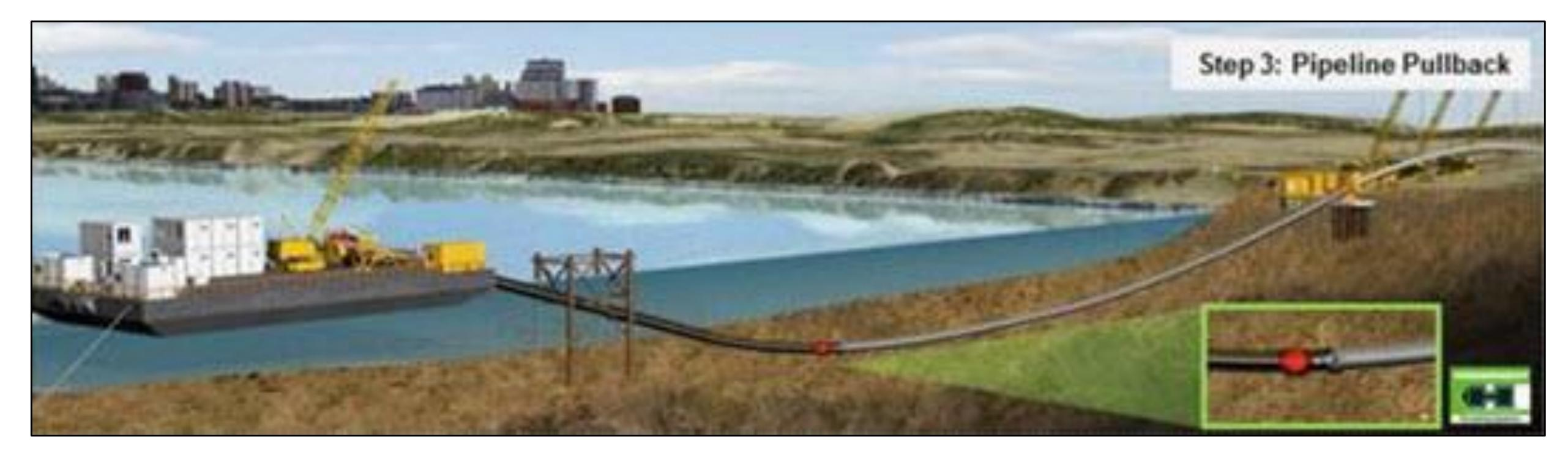
Pipeline Pullback - once the reaming process is complete and the pipe has been welded together, the pipe is pulled back through the boring site.
