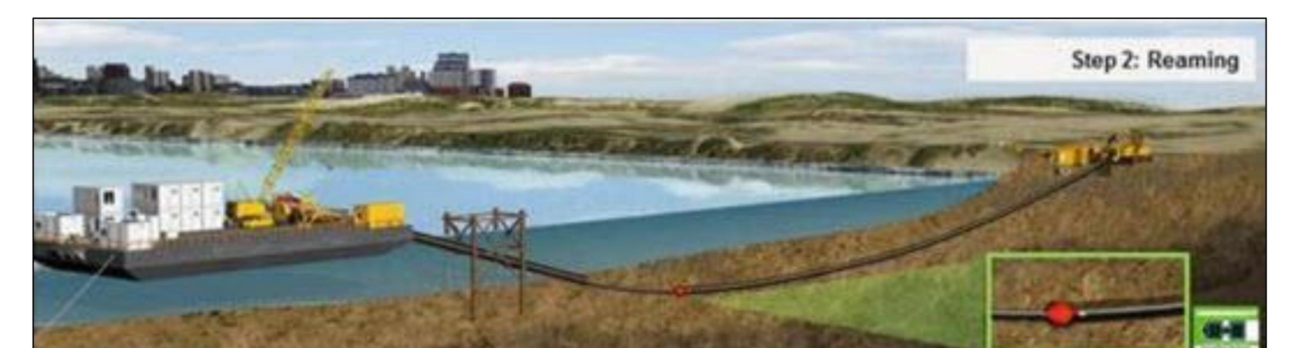
Reaming - the pilot bore's diameter is incrementally enlarged using reaming tools to drill from the exit site back to the entry point.
