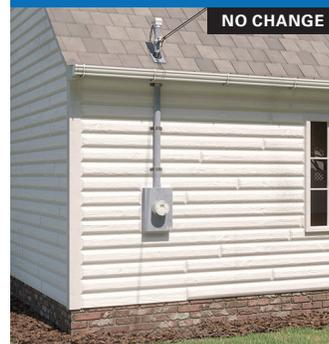
The electric line that serves the neighborhood would be placed underground, but the service line providing power to the house would remain overhead.
