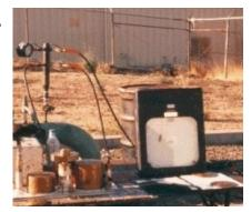
Pipeline is pressure tested to assure no defects exist. After the test, the pipeline is dried and cleaned.
