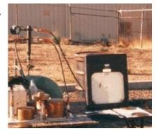
Pipeline is pressure tested to assure no defects exist. After the test, the pipeline is dried and cleaned.
