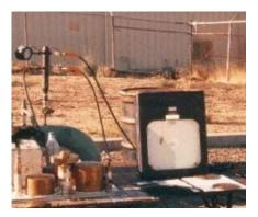
The newly constructed pipeline must be subjected to **pressure testing** before it can be placed into service. The purpose of a pressure test is to assure that no defects exist within the pipeline that might threaten its structural integrity. After the test, the pipeline is dried, cleaned and connected to the existing pipeline system.
