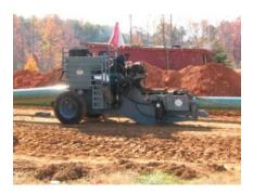
A **bending** machine is used to tailor the shape of the pipe to conform to the contours of the terrain or to make changes in the direction of the line.
