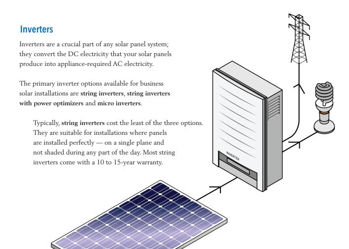
String inverters with power optimizers and micro inverters are more expensive, but are suitable for installations where one or more panels may be shaded, or where panels are installed on multiple planes and/or facing different directions. They also allow you to monitor the power production of each individual panel. Generally, warranties are 10 to 15 years for string inverters with power optimizers and 25 years for microinverters.
