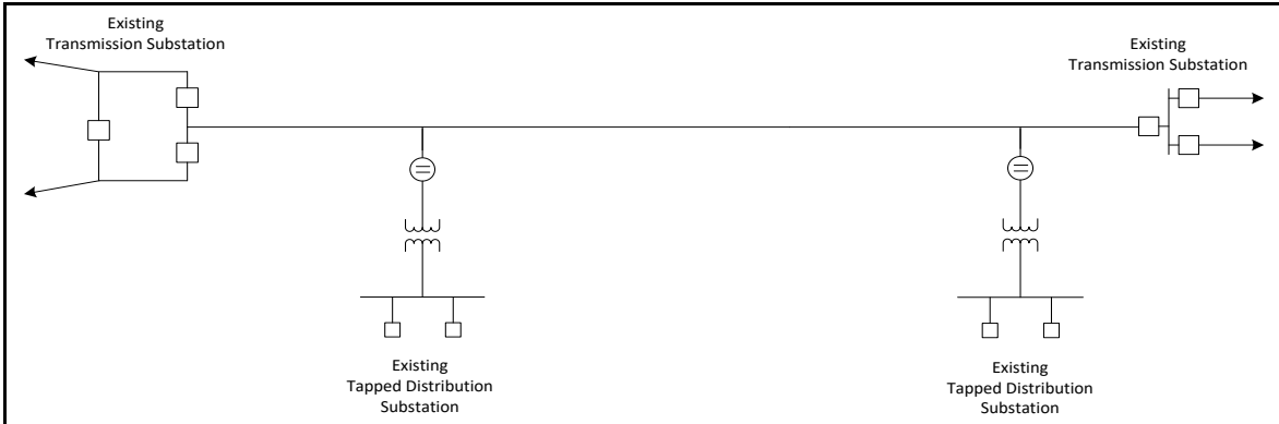
Figure 5. Existing Transmission Line
