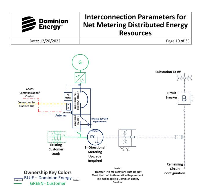
*Figure 3*: Typical Layout for Net Metering DER ≥250 kW and < 1,000 kW (DTT Required)
