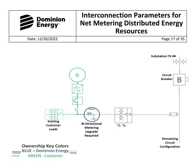
Figure 1: Typical Layout for Net Metering DER < 250 kW
