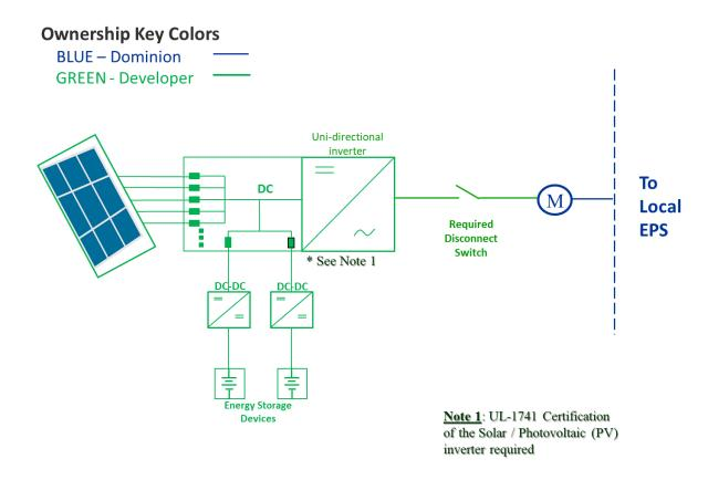
Figure 4: DC coupled ESS (Configuration 3)
